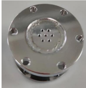
Figure 4. The orifice plate structure in the system to inhibit the superfluid helium crawling membrane
